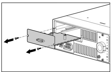
5. Install the SNMP / Serial Port Card. Take care to seat it properly.
